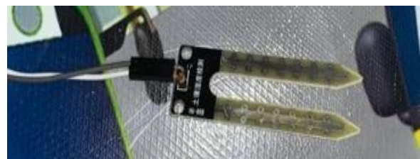
Gambar 4 Sensor Kelembaban Tanah
